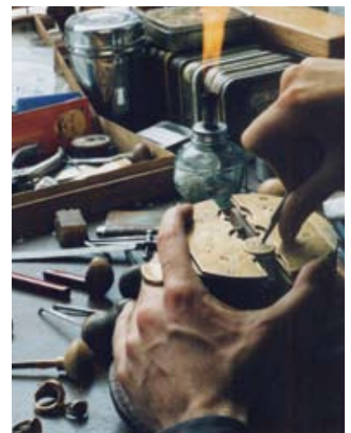
Working on a seal, cutting directly into the gold blank
